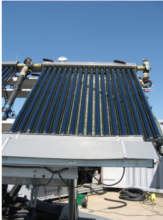
Figure 1: Picture of the collector SPA-58-1800-18-C mounted on the test facility of Fraunhofer ISE
